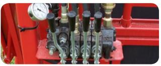
Convenient location of valve controls (Note: separate pressure controls for the neck extender).
