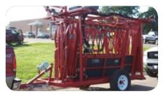
Portable Attachment balanced for easy positioning, the 2" x 4" steel frame with hand operated winch allows for one-man transport.
