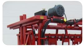
Features a 3 HP single-phase motor with vane pump for quiet operation, the power unit is isolated with rubber mounts and is easily relocated. (8 HP gas engine is available)
